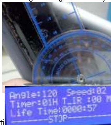
Figure 6. (a),(b),(c) Results of degree accuracy measurements For the accuracy measurement of the degree, additional testing is provided in a table for more completeness.
